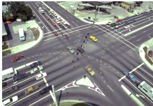
Exhibit 1-4. Signalized intersection with four approaches.
