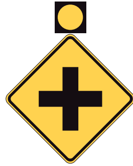
Figure 4 - MUTCD Examples of Enhanced Conspicuity for Signs (MUTCD, Section 2A.15)
