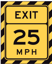
Figure 4 - MUTCD Examples of Enhanced Conspicuity for Signs (MUTCD, Section 2A.15)
