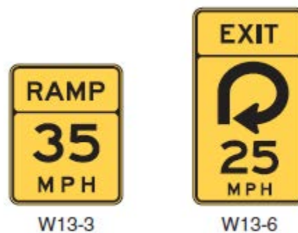
Figure 50. Ramp advisory speed limit signs (14).
