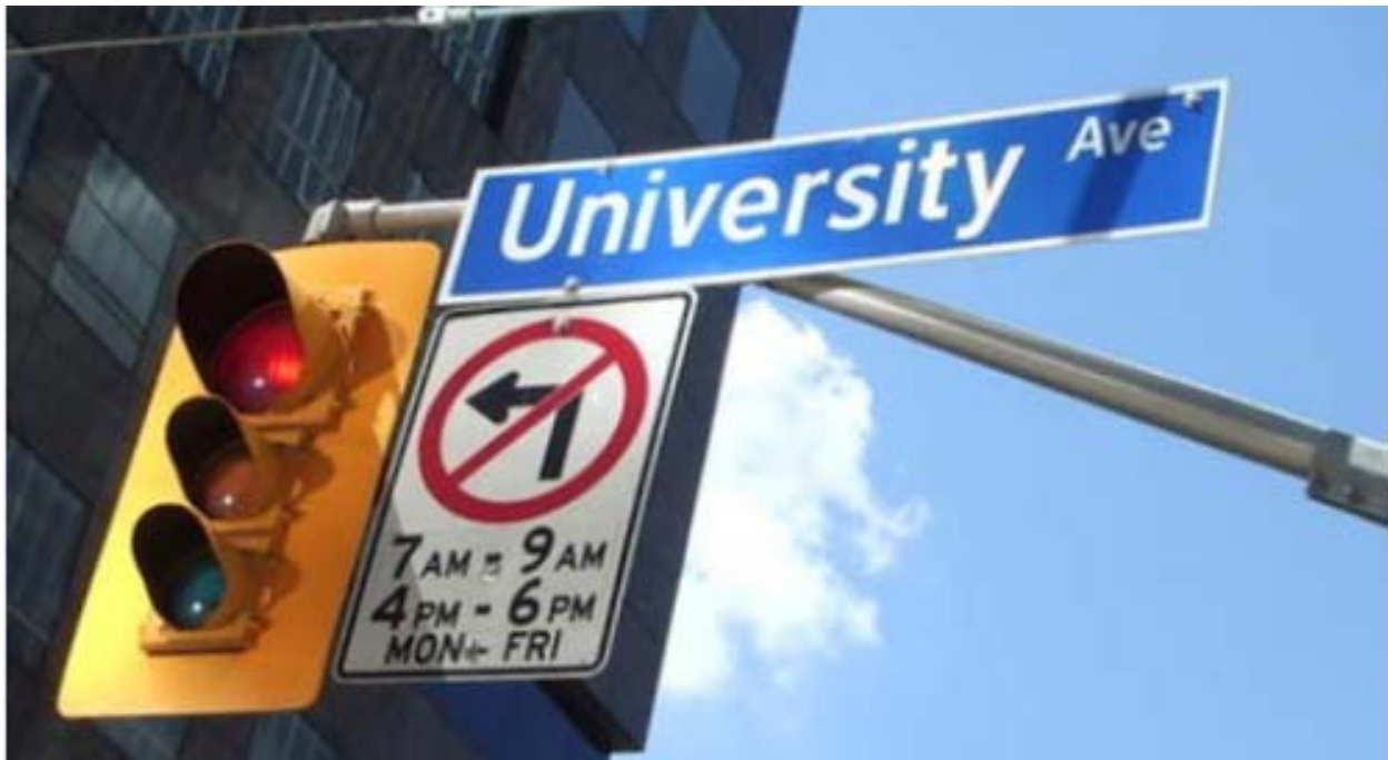
Figure 39. No left turn permitted during certain portions of the day (30).
