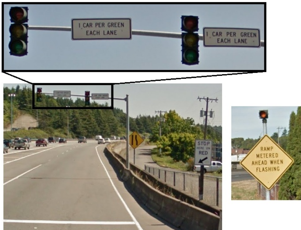
Figure 49. Presence of ramp metering (27).
