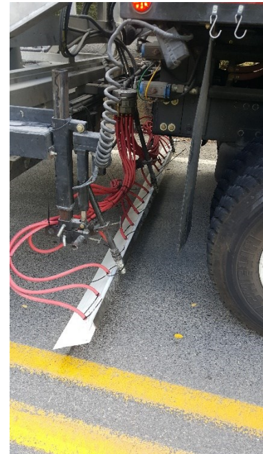
Figure 8: Equipment Associated with Fully-Automated Application. Source: PennDOT
