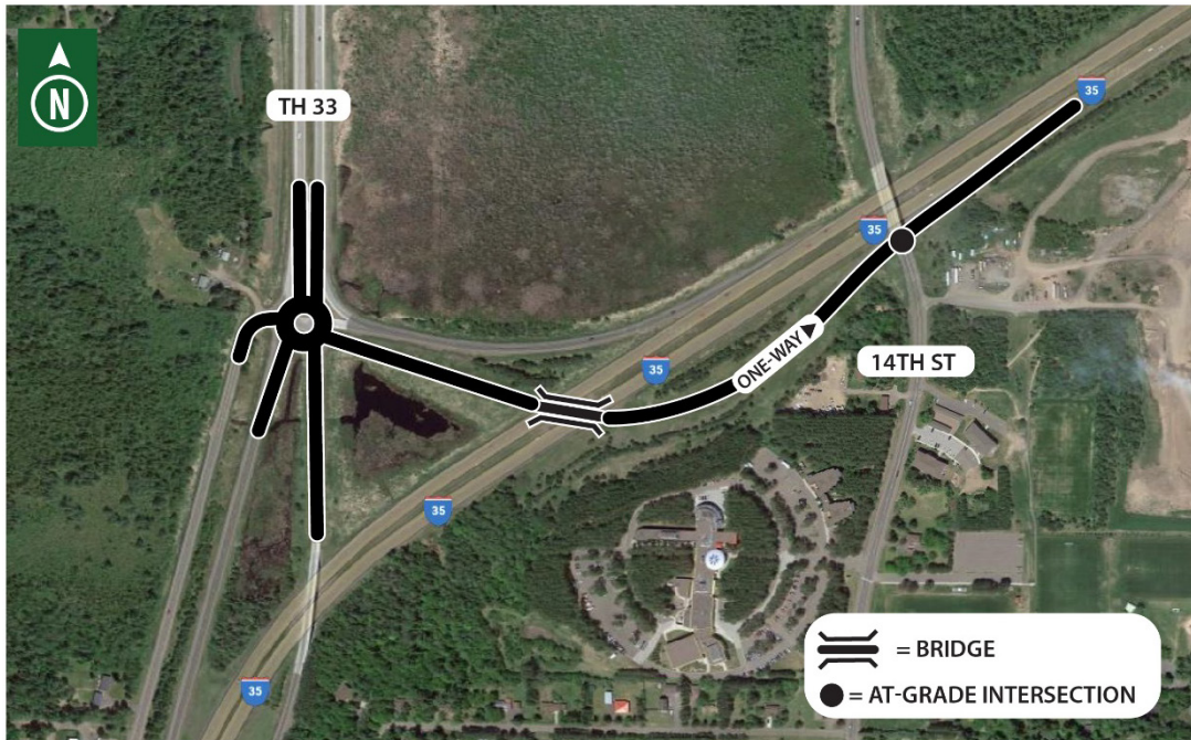
Figure 5. Graphic. Concept D Split Diamond with Eastbound Collector Distributor.
