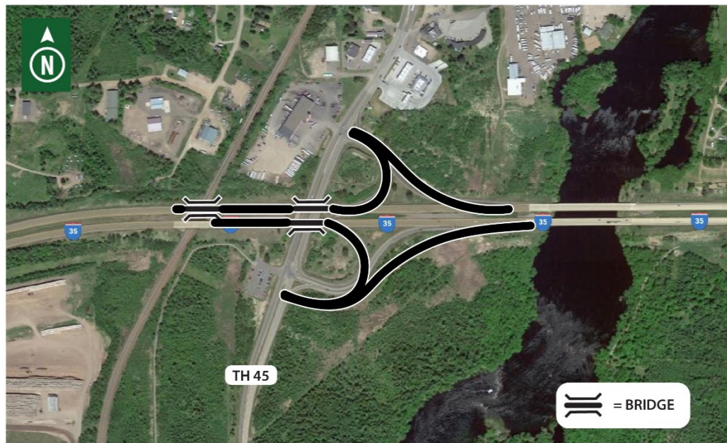
Figure 7. Graphic. Concept F Wider Bridges with Modified Ramps and Loops.
