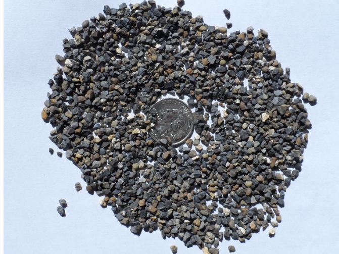
Figure 6. Photograph. Calcined bauxite aggregate for HFST.
