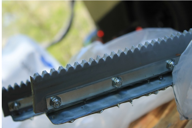
Figure 27. Photo. Example of spiked shoes worn by squeegee operator.
