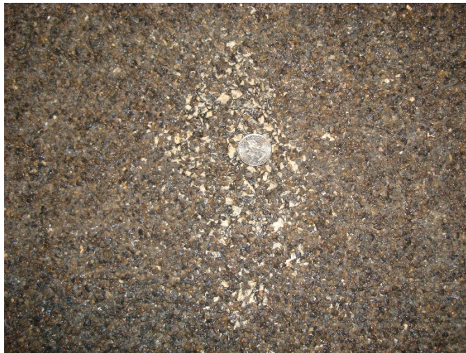
Figure 34. Photo. Example of exposure of underlying pavement after sweeping.
