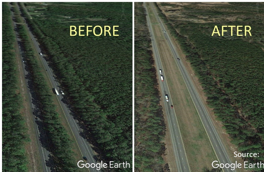
Figure 2: Clear Zone Reclamation along I-26
