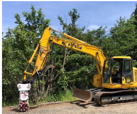
Excavator with grinder attachment
