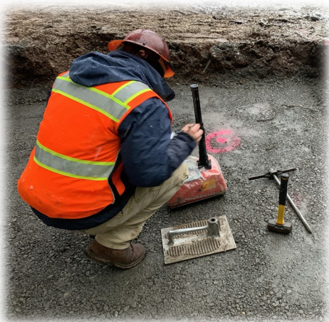
Below: Testing Compaction
