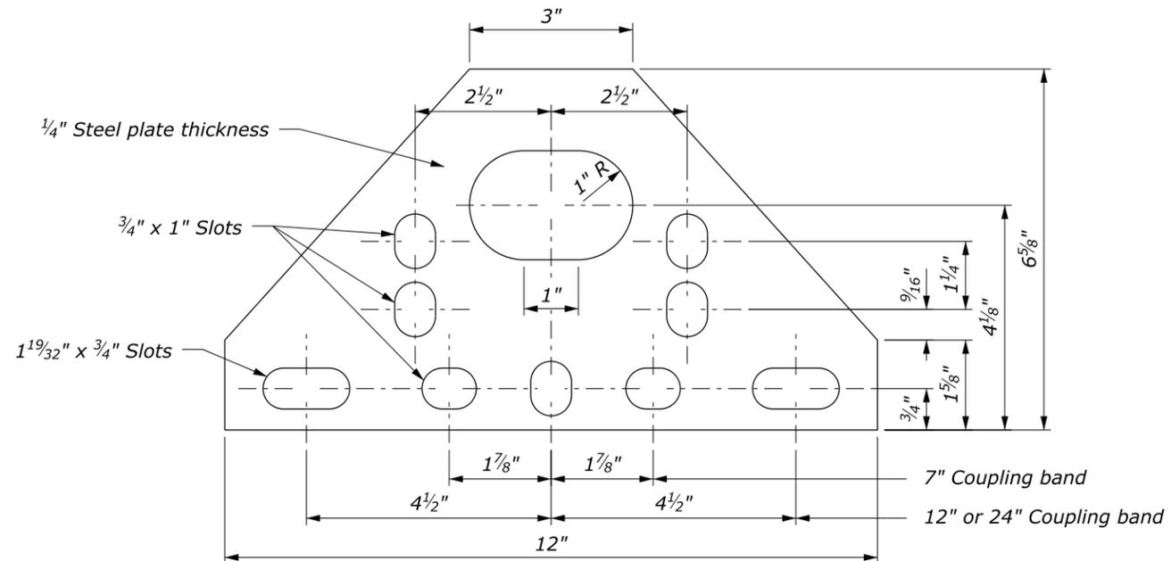
Measure length of coupling band parallel to the centerline of the pipe
