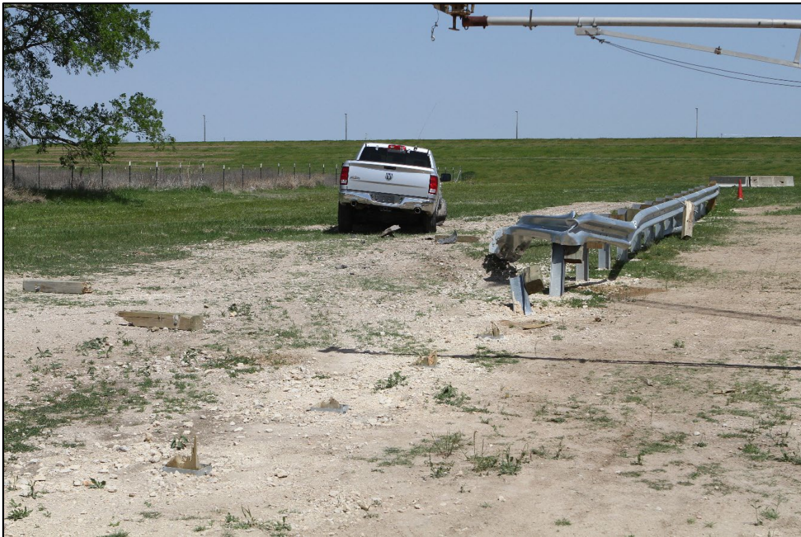
Figure 3.29. TL-2 Terminal on MGS Post Impact for Crash Test 615181-01-8.
