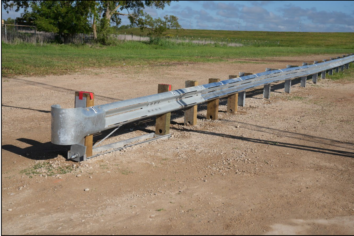
Figure 9.5. TL-2 Terminal on MGS prior to Crash Test 615181-01-7.
