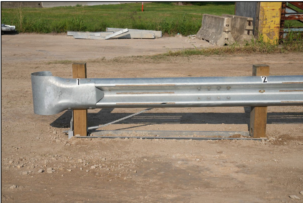
Figure 5.3. TL-2 W-beam End Terminal prior to Test 615181-01-5.
