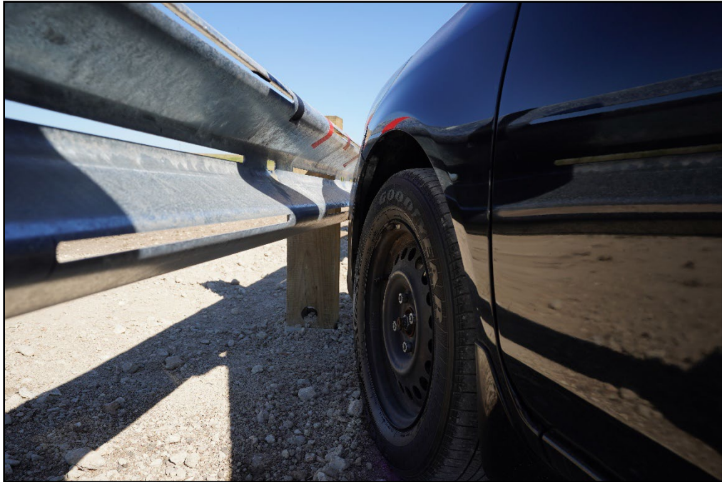
Figure 12.2. TL-2 W-beam End Terminal/Test Vehicle Impact Location 615181-01-13.
