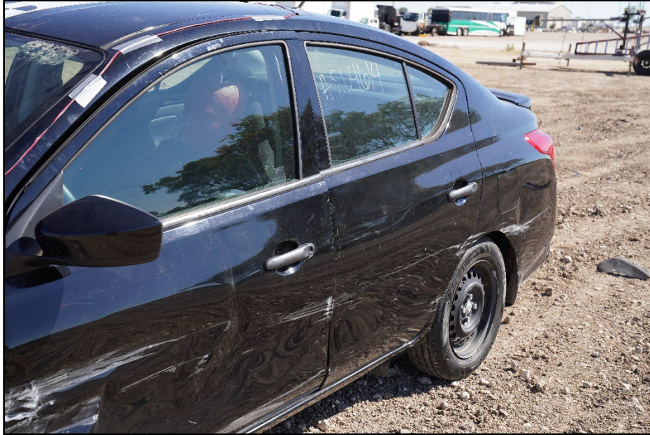
Figure 12.8. Rear Impact Side of Test Vehicle after Test 615181-01-13.
