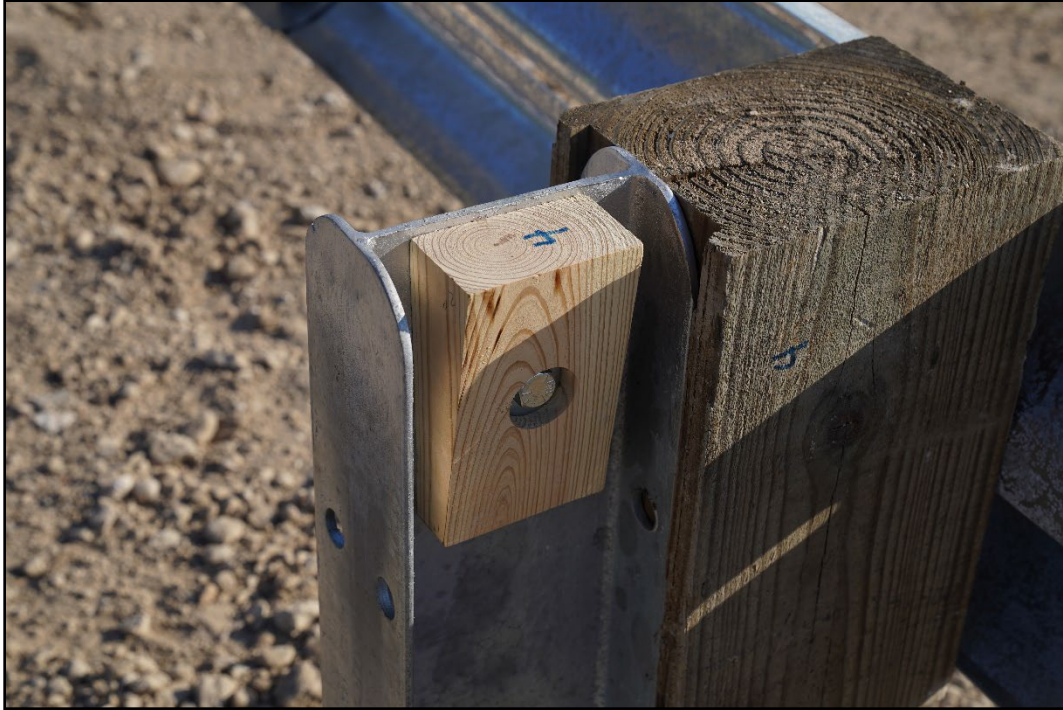
Figure 5.11. TL-2 W-beam End Terminal on the Impact Side of Post 4 prior to Tests 615181-01-11 & 615181-01-12.
