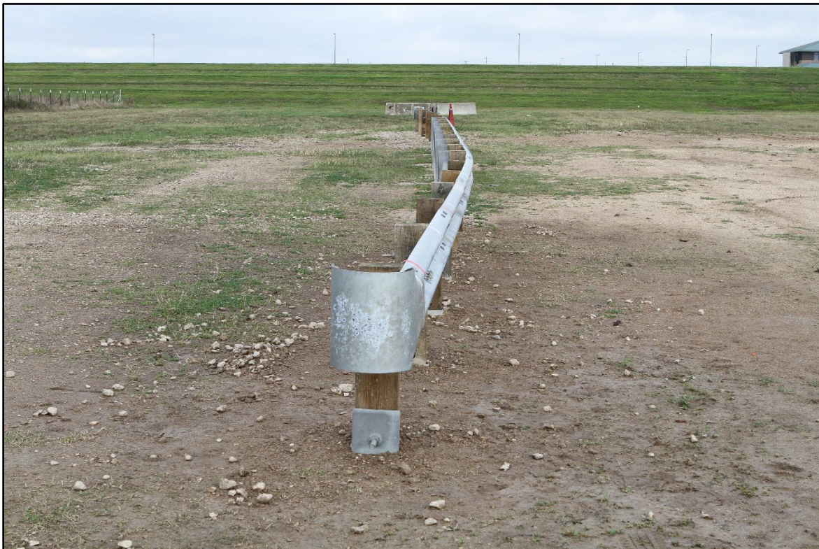
Figure 3.16. In-Line View of the TL-2 Terminal on MGS prior to Crash Test 615181-01-10.
