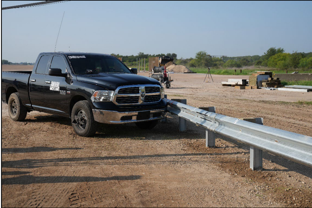
Figure 8.1. TL-2 W-beam End Terminal/Test Vehicle Geometrics for Test 615181-01-5.
