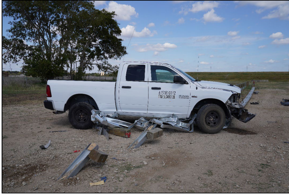
Figure 11.5. TL-2 W-beam End Terminal after Test at Impact Location 615181-01-12.
