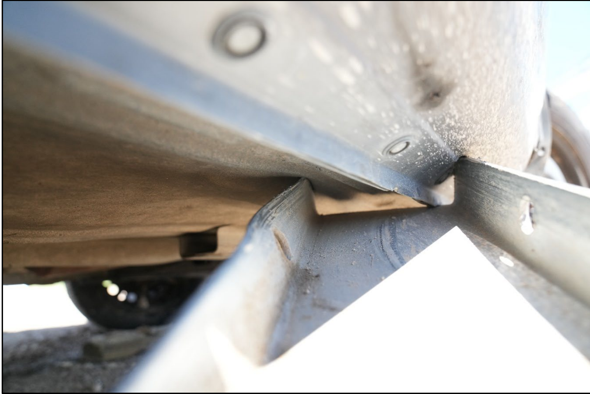
Figure 9.8. Post Engaged with Undercarriage of Vehicle after Crash Test 615181-01-7.
