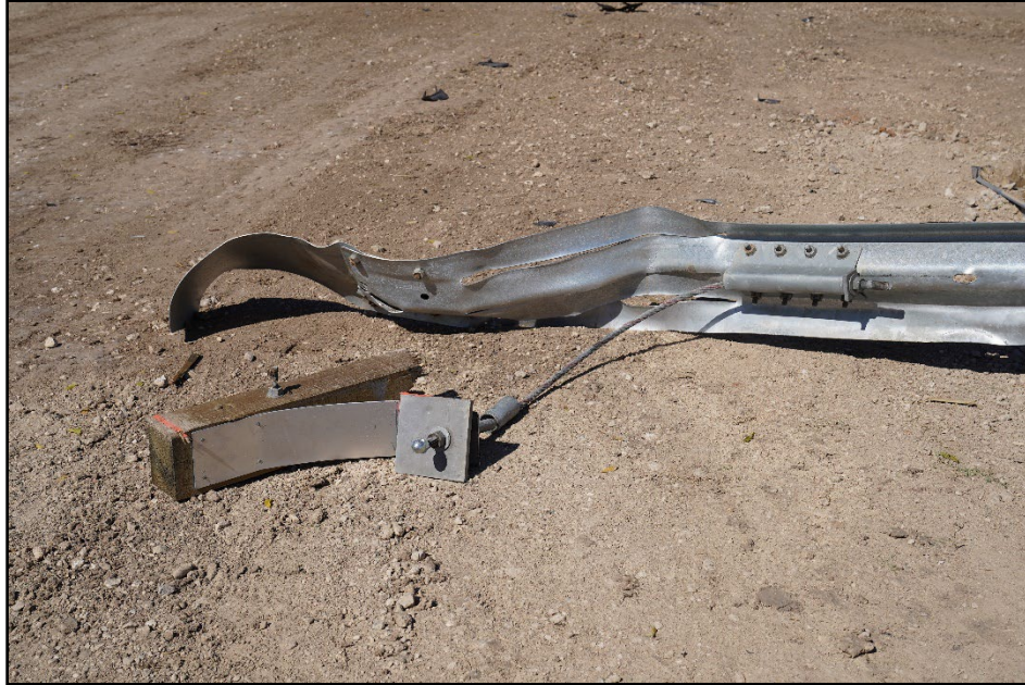
Figure 12.6. End of the Rail and Anchor Post of the TL-2 W-beam End Terminal after Test 615181-01-13.
