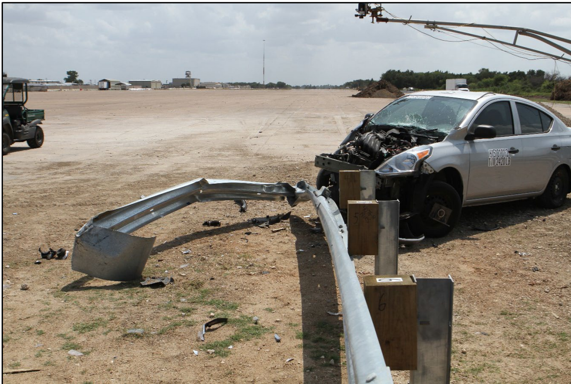
Figure 3.10. TL-2 Terminal on MGS Post Impact for Crash Test 615181-01-2.
