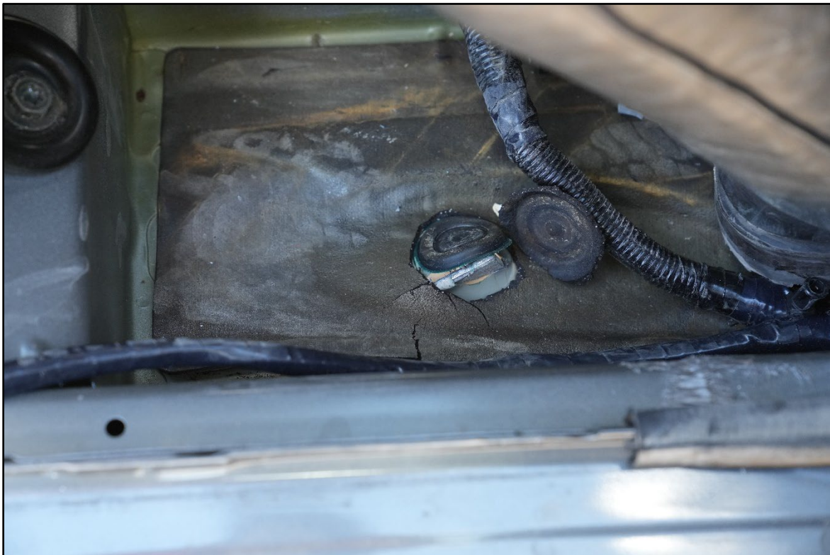
Figure 9.9. Occupant Compartment Damage after Crash Test 615181-01-7.
