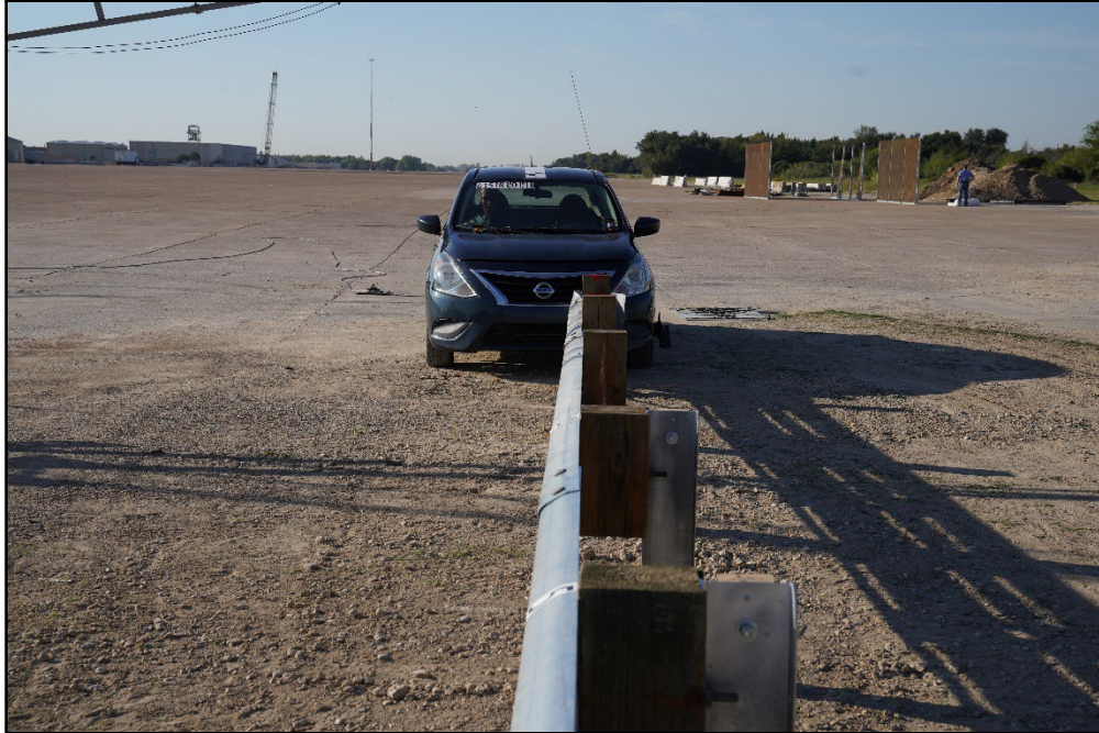
Figure 10.1. TL-2 W-beam End Terminal/Test Vehicle Geometrics for Test 615181-01-11.
