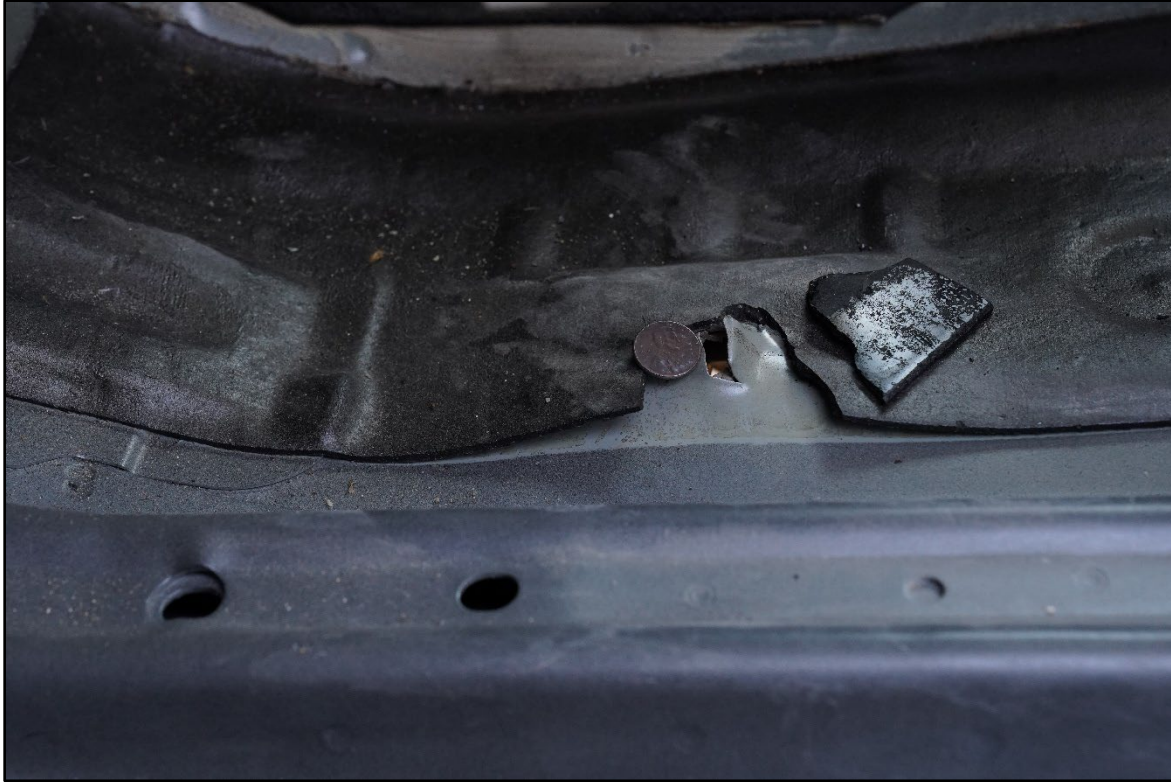
Figure 9.2. Occupant Compartment Penetration after Crash Test 615181-01-6.
