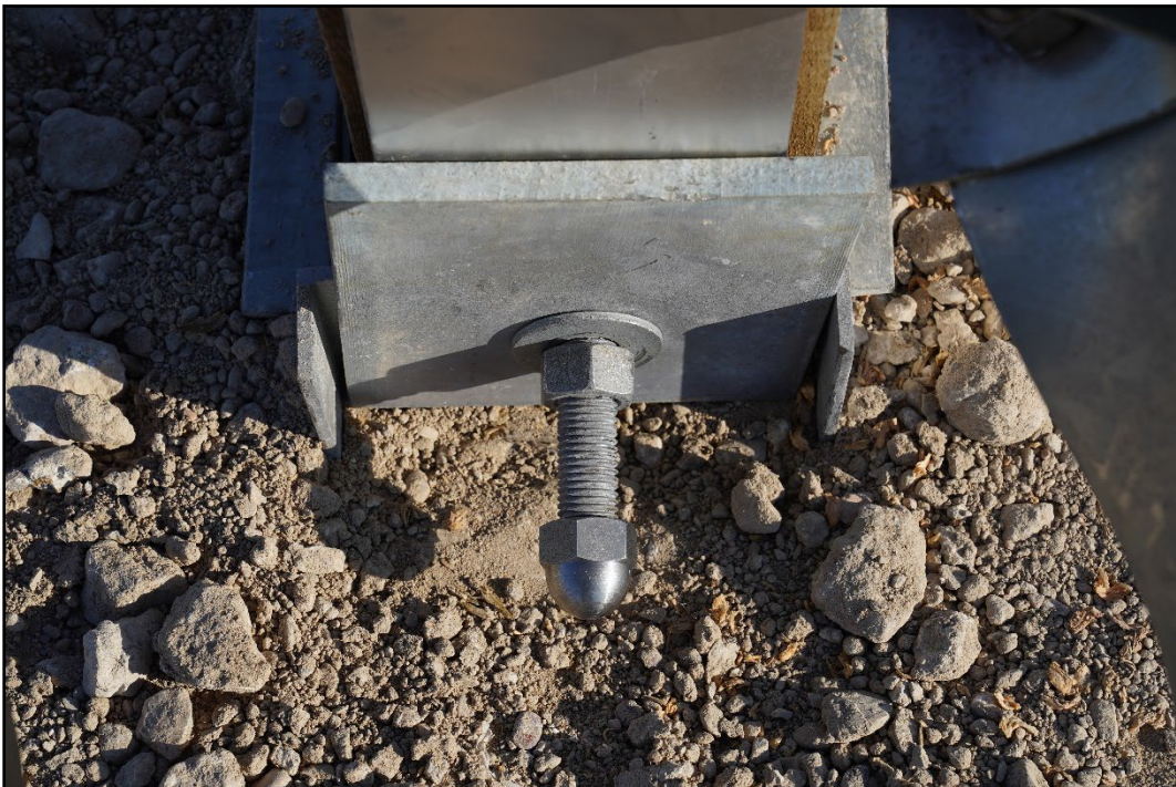
Figure 5.10. The Anchor Bolt with Cap Nut on the TL-2 W-beam End Terminal prior to Tests 615181-01-11 & 615181-01-12.
