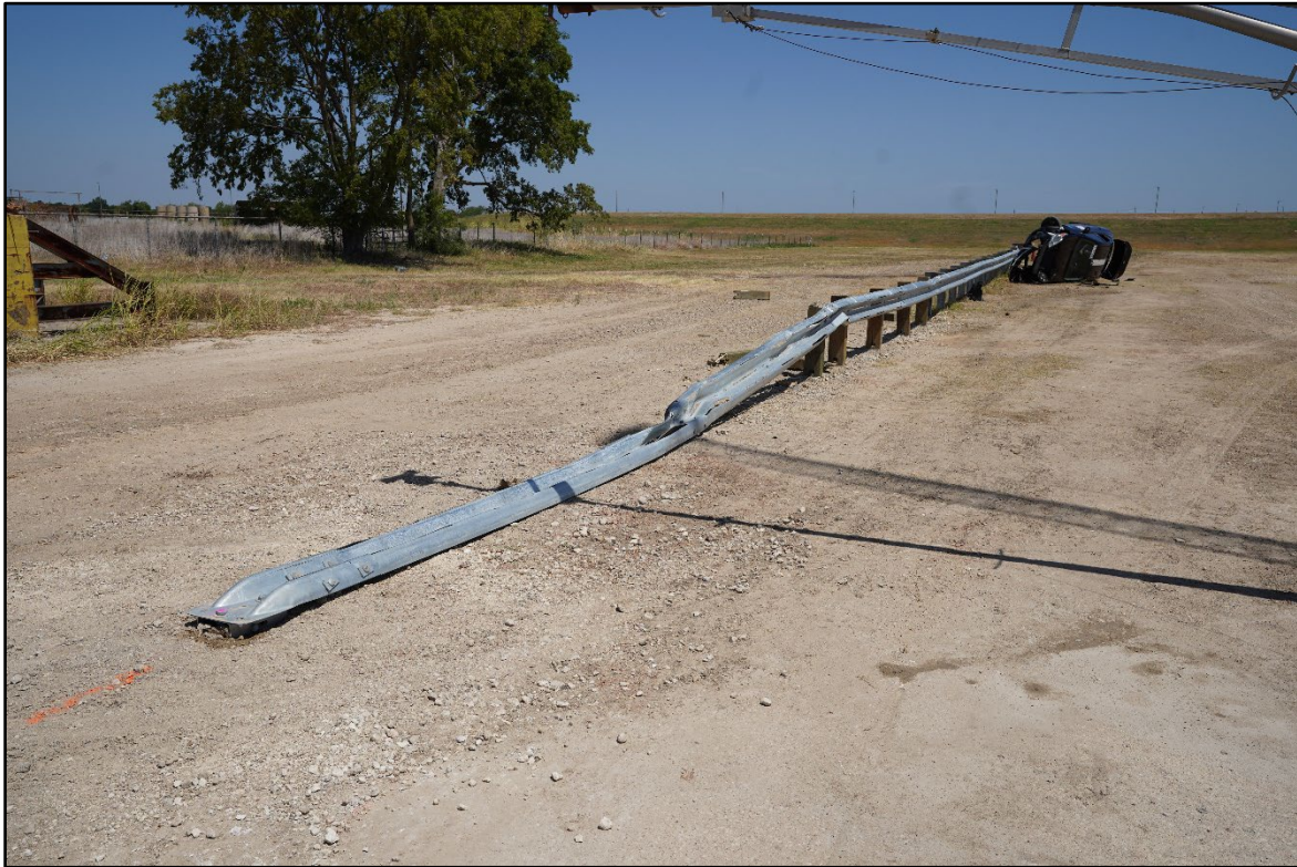
Figure 3.33. TL-2 Terminal on MGS Post Impact for Crash Test 615181-01-3.
