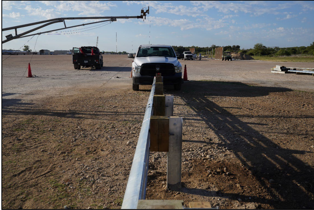
Figure 11.1. TL-2 W-beam End Terminal/Test Vehicle Geometrics for Test 615181-01-12.
