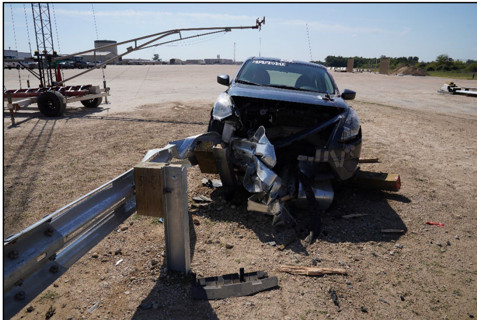
Figure 10.5. TL-2 W-beam End Terminal after Test at Impact Location 615181-01-11.
