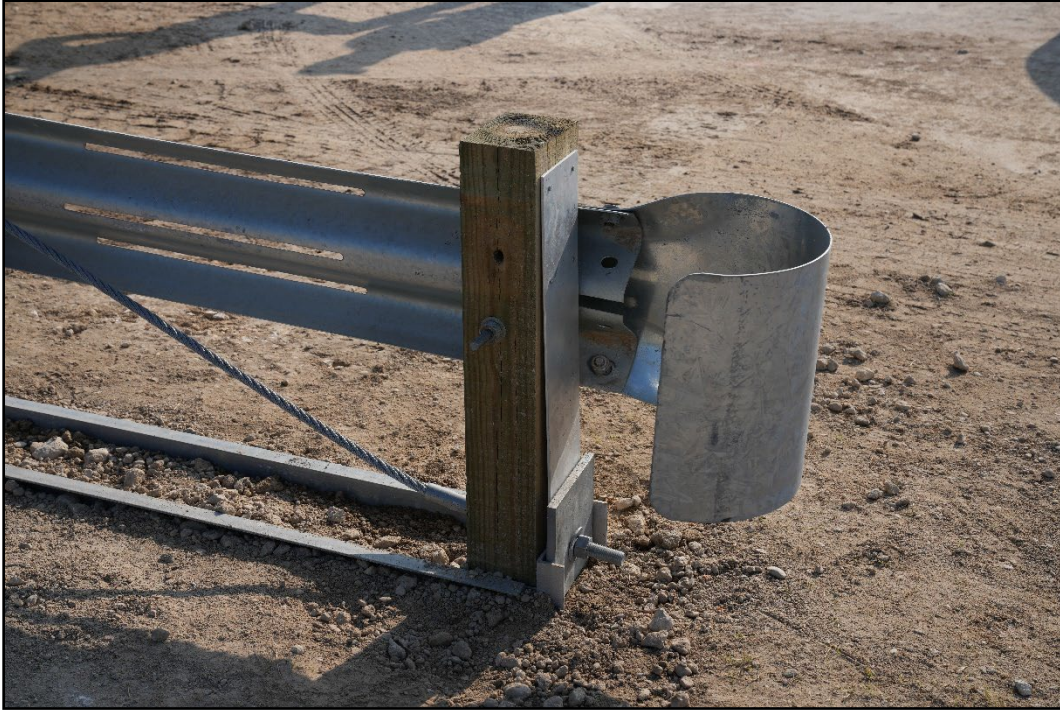
Figure 5.6. Field Side of the TL-2 W-beam End Terminal prior to Test 615181-01-5.
