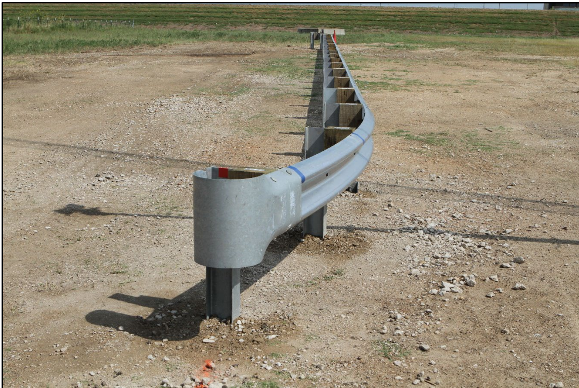
Figure 3.9. In-Line View of the TL-2 Terminal on MGS prior to Crash Test 615181-01-2.
