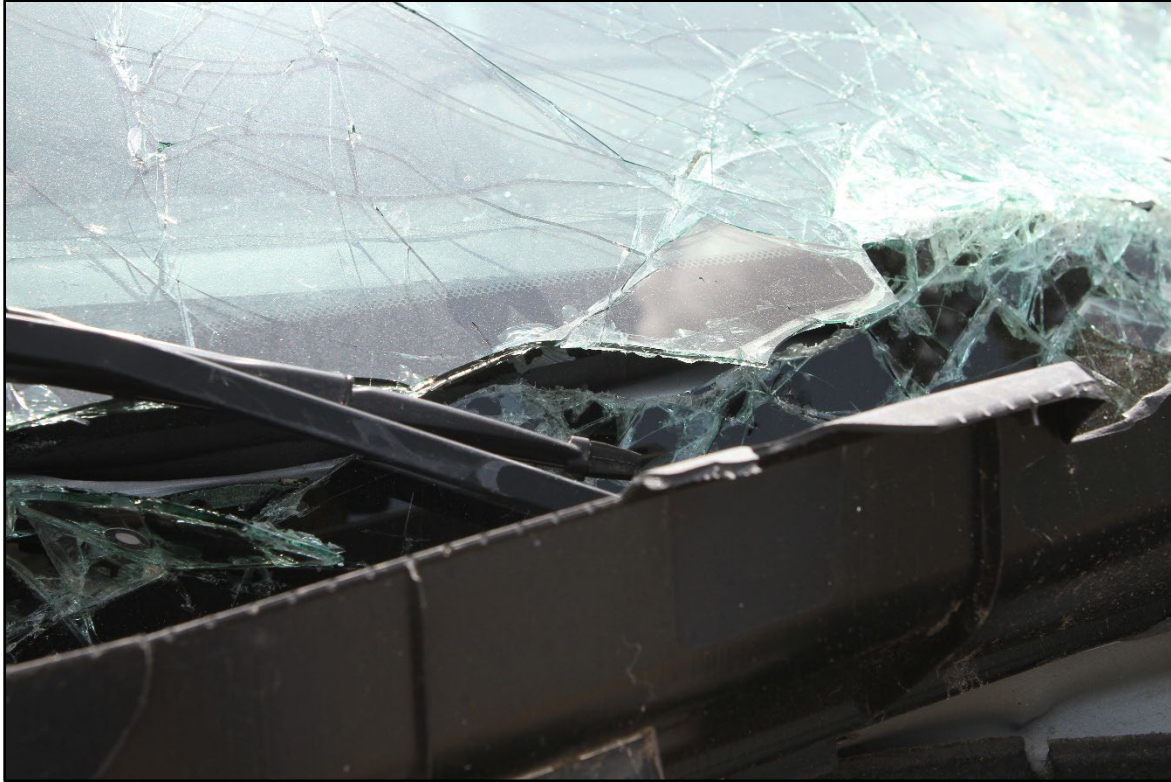
Figure 3.11. Detailed View of the Windshield after Crash Test 615181-01-2.
