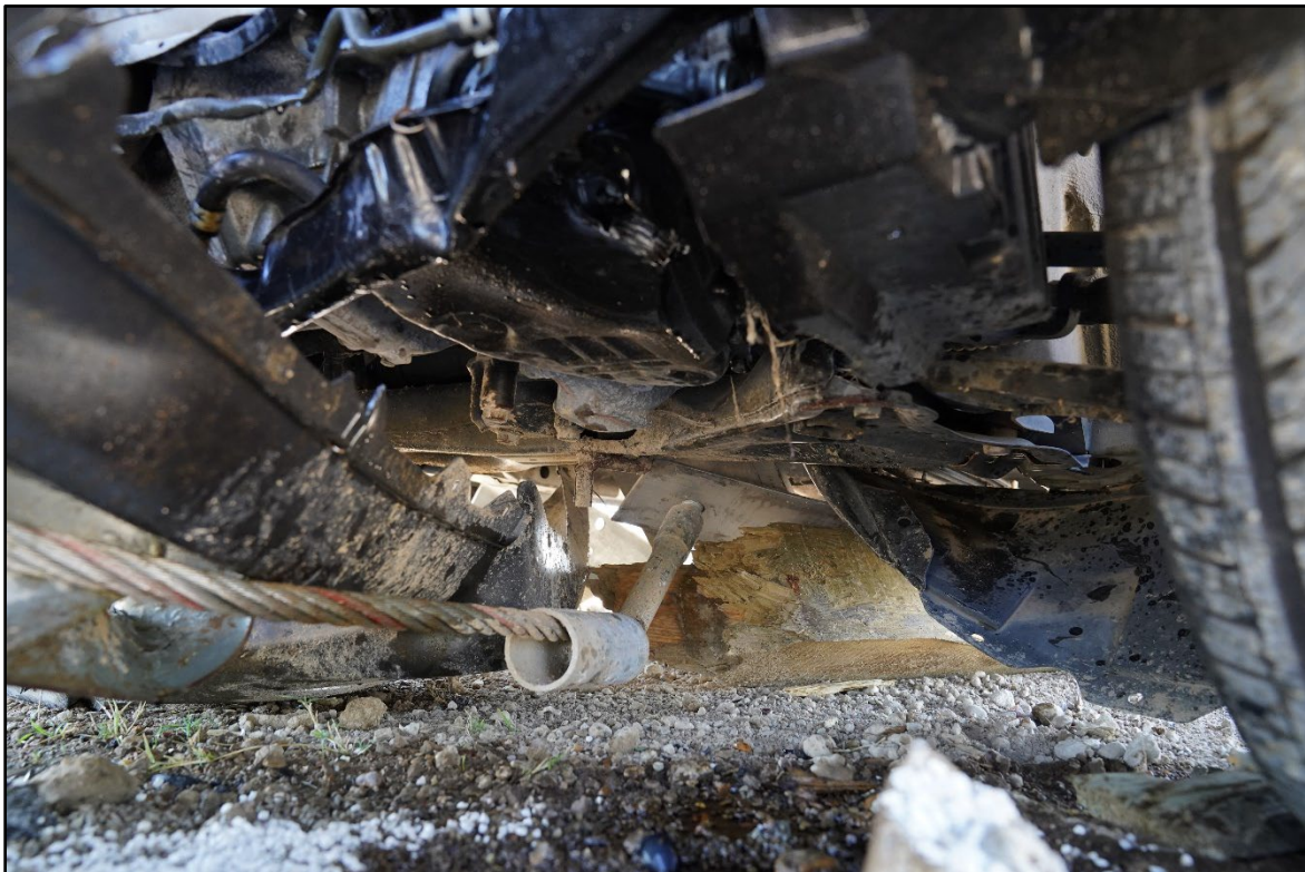
Figure 9.3. Undercarriage Damage after Crash Test 615181-01-6.
