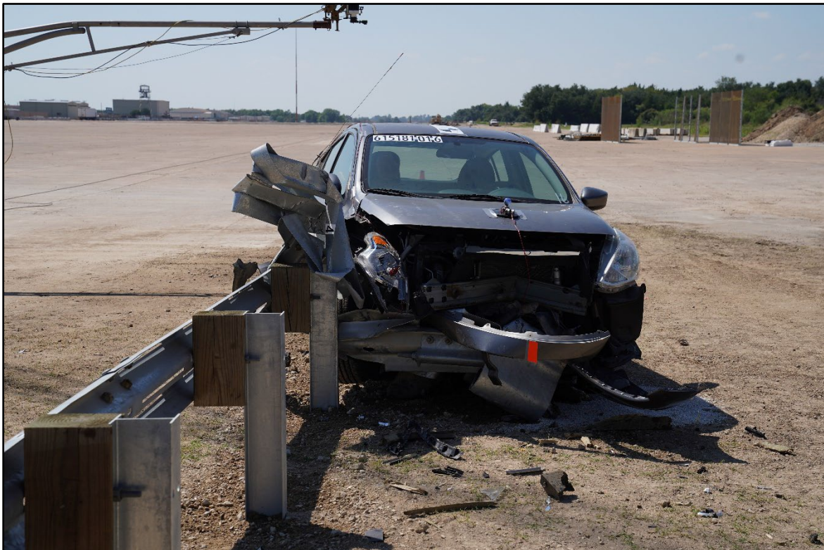
Figure 9.1. TL-2 Terminal on MGS Post Impact for Crash Test 615181-01-6.
