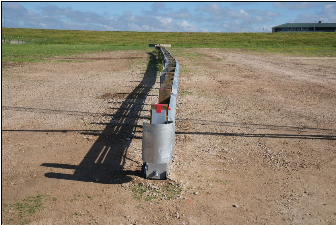
Figure 9.6. In-Line View of the TL-2 Terminal on MGS prior to Crash Test 615181-01-7.
