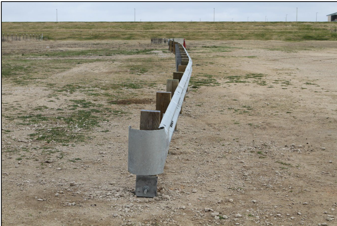
Figure 3.23. In-Line View of the TL-2 Terminal on MGS prior to Crash Test 615181-01-9.
