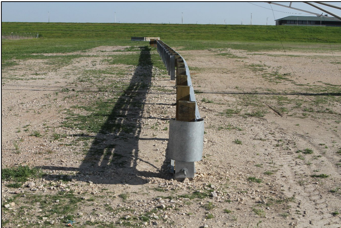
Figure 3.28. In-Line View of the TL-2 Terminal on MGS prior to Crash Test 615181-01-8.
