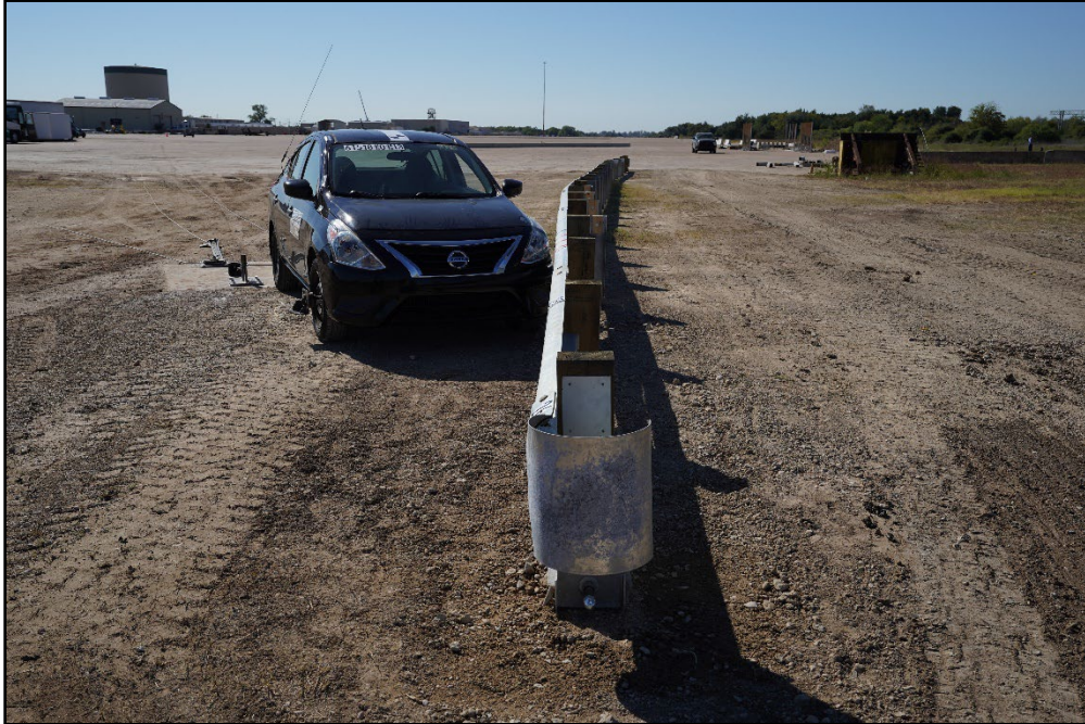
Figure 12.1. TL-2 W-beam End Terminal/Test Vehicle Geometrics for Test 615181-01-13.
