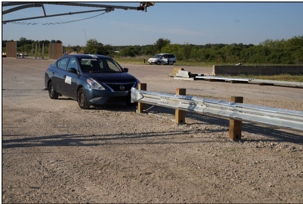
Figure 10.2. TL-2 W-beam End Terminal/Test Vehicle Impact Location 615181-01-11.
