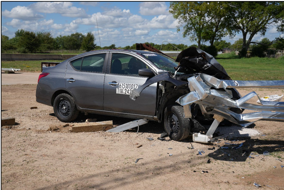
Figure 9.7. TL-2 Terminal on MGS Post Impact for Crash Test 615181-01-7.
