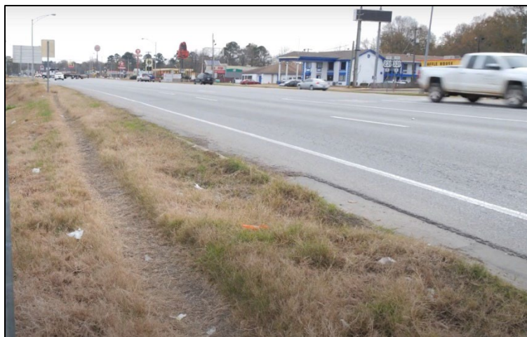
Figure 50. Photograph. Example of an informal desire path created by pedestrians. (63)
