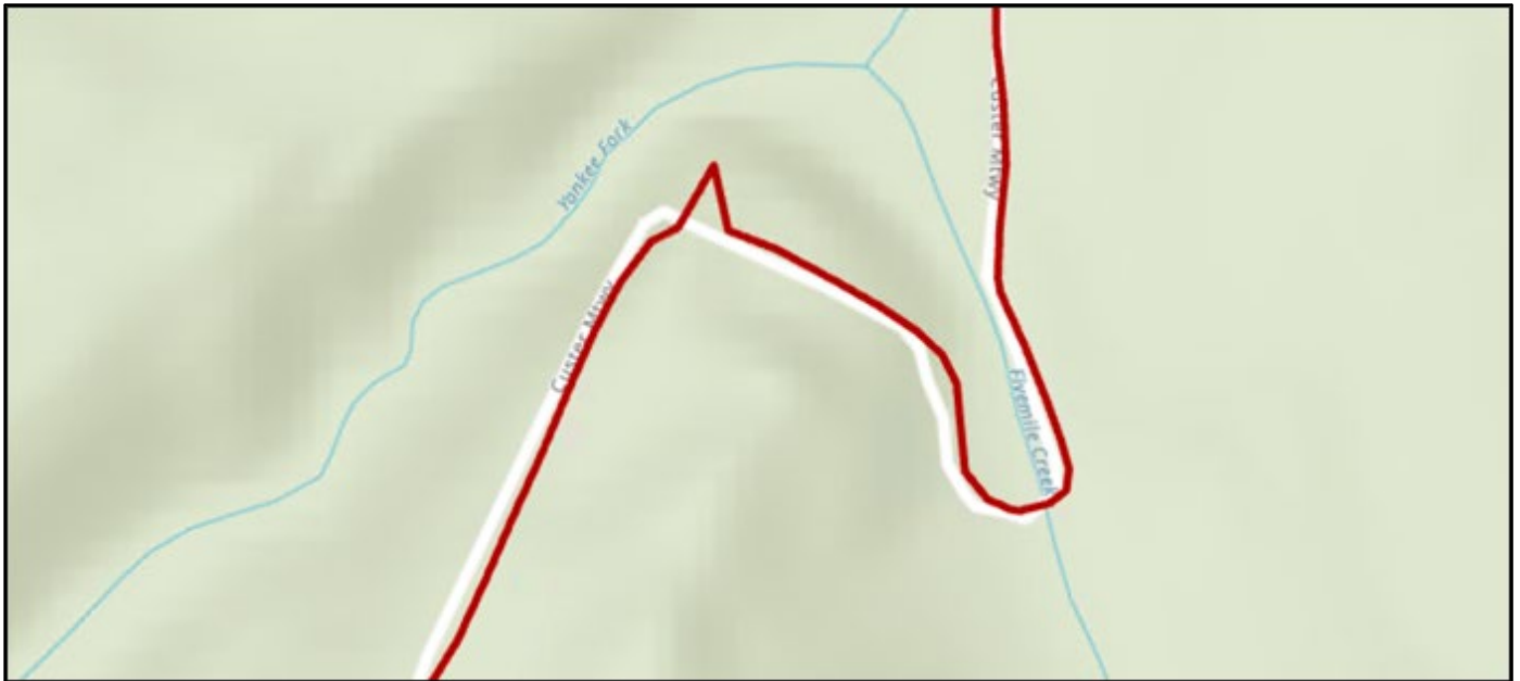
Figure 13. Graphic. Example of a harsh angle in centerline geometry.
