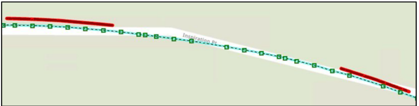
Figure 14. Graphic. Example of closely spaced vertices along a curve.
