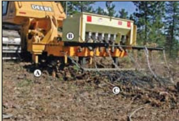
**Figure 10.91** – Seed sowing and mixing equipment can be attached to most types of ground based equipment, including all-terrain vehicles. A seed spreader attached to the back of an all-terrain vehicle broadcasts seeds on the soil surface and a chain harrow mixes seeds into the soil.
