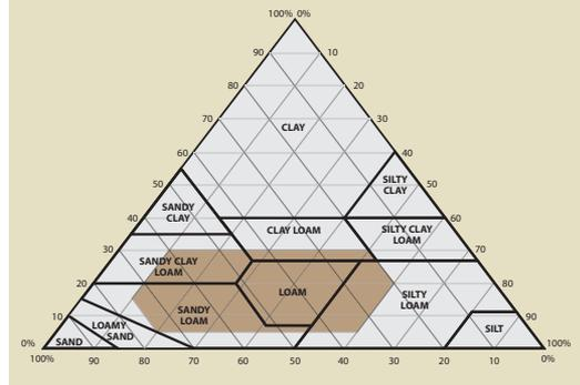
**Table 10.6** – General specification ranges for loam borrow used in manufactured topsoil. These can be modified depending on the soil characteristics of the compost and other soil amendments (modified after Alexander 2003b; CCREF and USCC 2006).
