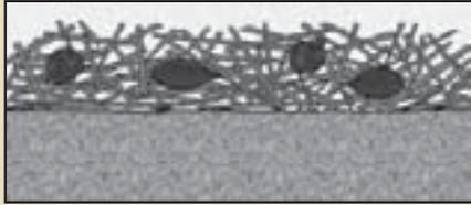
**Figure 10.95** – Applying seeds in a hydromulch places a portion of seeds on the soil surface and some suspended in the hydroseeding matrix above the surface.
