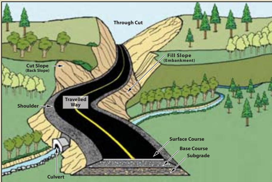
Figure 3.7 – Terms used to define roads: cross-section.
