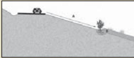
**Figure 5.5** – Planting pockets are designed to capture water from upslope runoff (A), that collects in a slight depression (B). Captured water wets up the soil after each rainstorm and drains into the fractured bedrock (C). Soil is protected from surface erosion on the downhill side of the pocket with mulch or erosion fabric (D).
