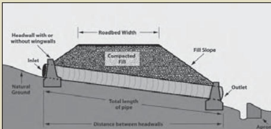
**Headwall** – A concrete, gabion, masonry, or timber wall built around the inlet or outlet of a drainage pipe or structure to increase inlet flow capacity, reduce risk of debris damage, retain the fill material, and minimize scour around the structure.
