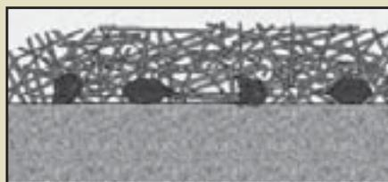
**Figure 10.94** – Seeds mixed into long-fibered mulch have less contact with soil, which can reduce germination.
