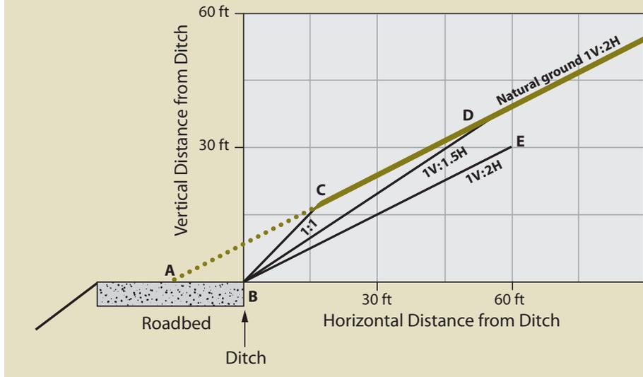
for soil erosion is considerably reduced. Furthermore, there is a substantial cost savings with less excavation and revegetation work. Figure 5.51 gives an example of how increasing the steepness of a cut slope on a typical 1V:2H natural ground slope substantially decreases the length of disturbed soils.
