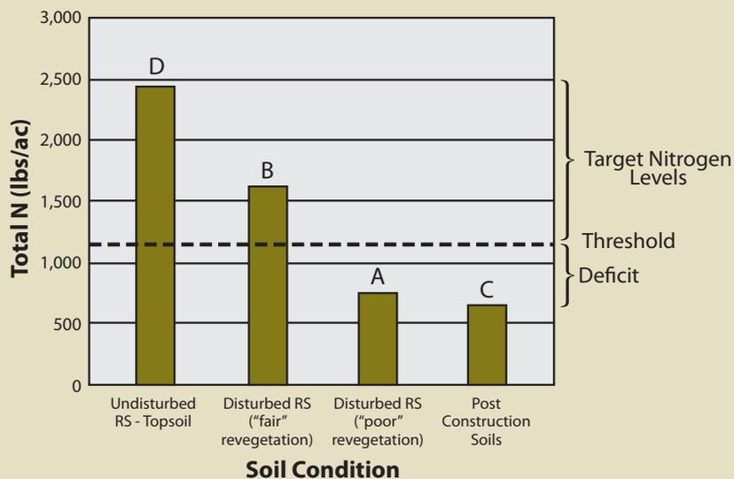
**Figure 10.2** – Determining the amount of nitrogen (N) needed to bring soils up to a nitrogen threshold can be calculated from equations shown in this spreadsheet.
