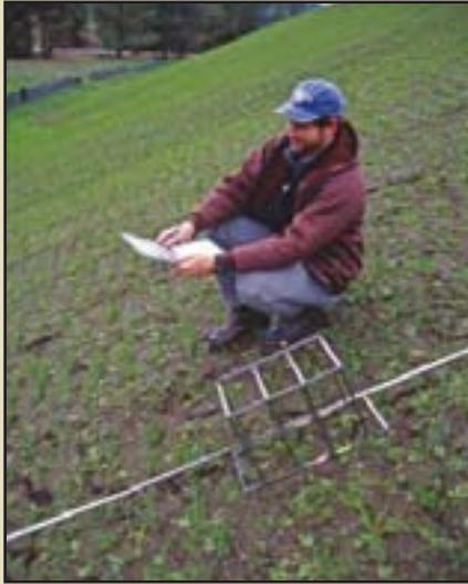
**Figure 12.3** – A fixed frame can be adapted to allow for the positioning of a laser pointer at 20 points in the frame. Soil cover or plant cover attributes are recorded at each laser point. The frame in this example is 8 in by 20 in, with 2 in spacing within rows and 4 in spacing between rows. The laser is a Class IIIa red laser diode module that produces a 1mm dot.
