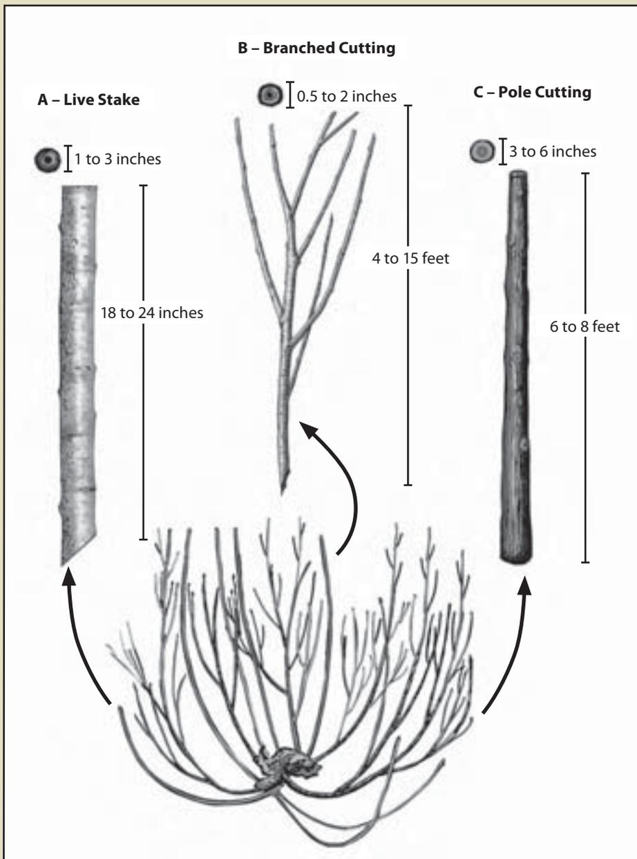
sections of second- or third-year wood. Live stakes are typically 18 to 24 inches in length and from 1 to 3 inches in diameter (Figure 10.73A). Depending on the plant species, it can take 2 to 4 years for a stooling bed to produce large enough branches for live stakes. Some of the smaller willow species will never grow large enough.
